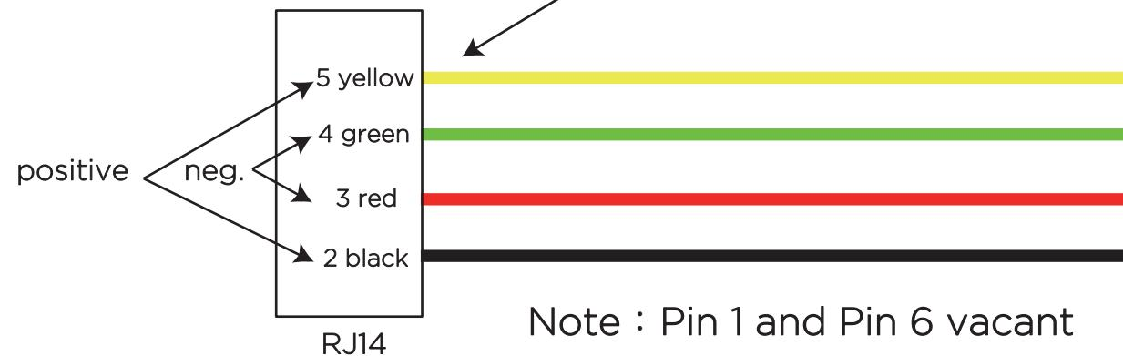
Definition for controller and ballast connection RJ14
