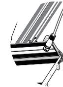
**3** Once all the LED bars are fastened into place and A/C cables are attached to the mast, turn the fixture over (this may require more than one person). Ensure the flat surface is clear of anything that could damage the delicate diodes.
