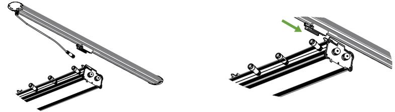
**2** Once the plastic clips are all snapped in place, attach the A/C cables coming from the mast to each LED bar by aligning the connector pins and pressing the ends together. Lock by twisting in opposite directions.
