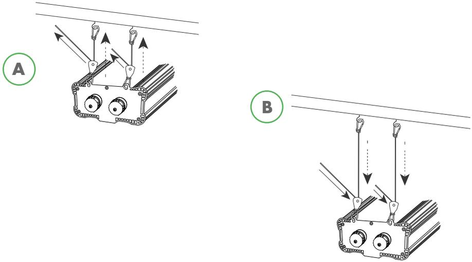
**2** Lift the LED and attach the carabiners to pre-installed hooks from ceiling or mounting beam. The Ratchets should be installed closest to the LED (and not the ceiling).
