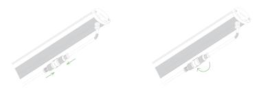
Once all the LED bars are fastened into place and A/C cables are attached to the mast, turn the fixture over (this may require more than one person). Ensure the flat surface is clear of anything that could damage the delicate diodes.
