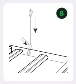
**3.** Once fixture is hanging with all LED bars installed, connect the power cable (blue tip) from the outlet to one side of the fixture.
